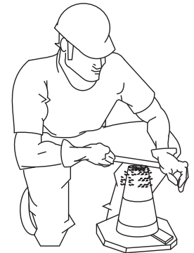
Figure 68-D. Slump Test (Removing Excess Concrete)
